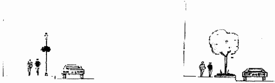
Figures 1 & 2: Examples showing various techniques to provide horizontal separation between pedestrian and vehicular traffic.
