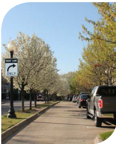
Slip streets, such as this one along Blackburn, slow traffic adjacent to the pedestrian zone.
