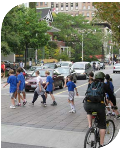
A speed table will encourage drivers to slow down and be more alert to pedestrians and bicyclists.
