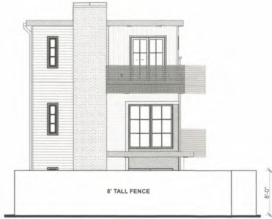
1 FENCE ELEVATION CARROLL SCALE : 3/32" = 1'-0"
