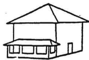
HIPPED ROOF, SYMMETRICAL, NO FRONT ENTRY
