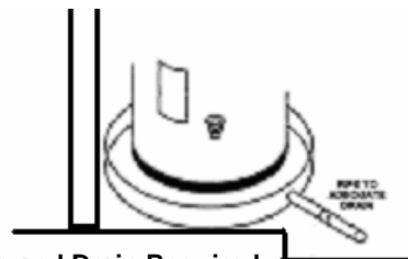
Pan and Drain Required Fig.2
