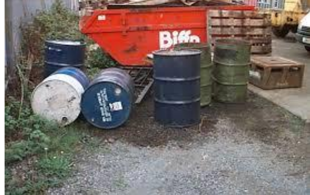
Figure 2 Drums not stored with containment.
