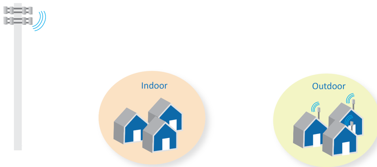
Figure 97: Sample Indoor and Outdoor Customer Antenna Configurations for a Fixed Wireless Network
