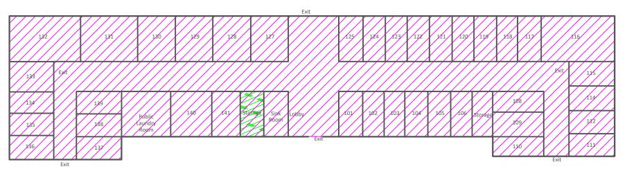
All Wallboard Walls and Ceiling Systems are Asbestos Containing Material (ACM) throughout
