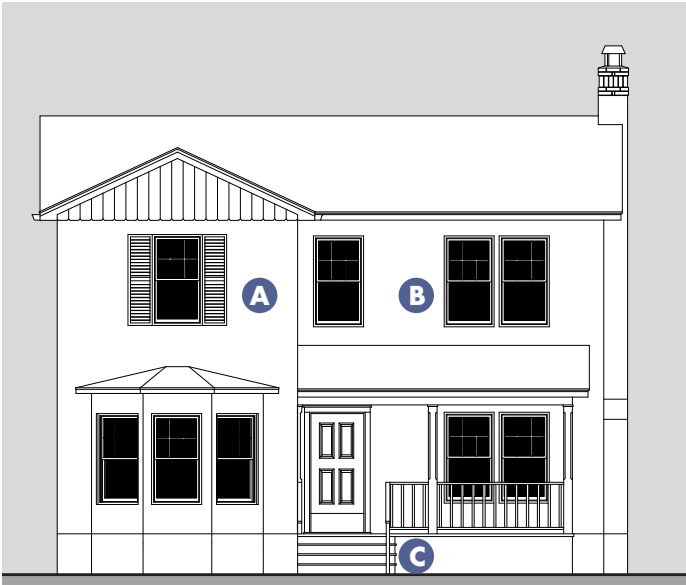
Example of smooth 3-coat stucco with bay window and front porch
