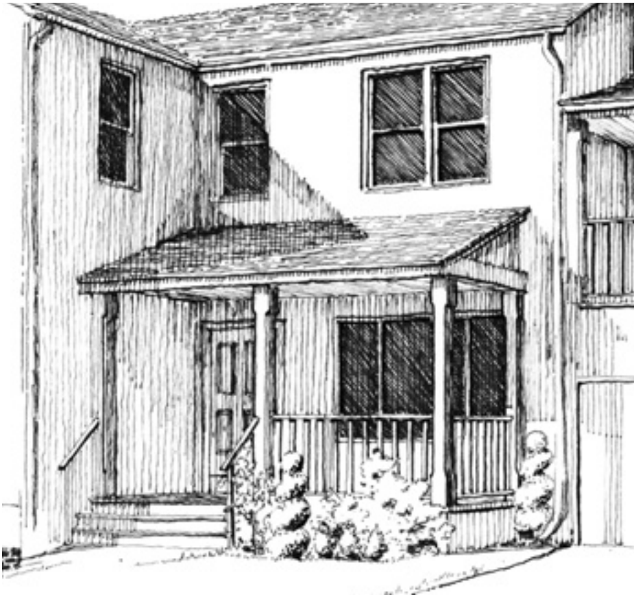
Crawl space vents: vertical slats
