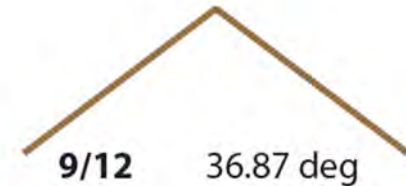
Examples: Diagrams showing minimum 5/12 and maximum 9/12 roof pitches for main roof.
