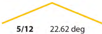
Examples: Diagrams showing minimum 5/12 and maximum 9/12 roof pitches for main roof.
