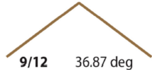
Examples: Diagrams showing minimum 5/12 and maximum 9/12 roof pitches for main roof.
