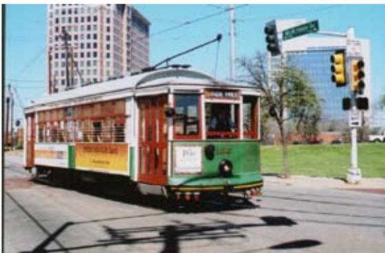
Streetcars are designed for local transportation and are most successful when tied into the local transit system. These transit vehicles are powered by overhead electricity and streetcar models range from modern to historic.
