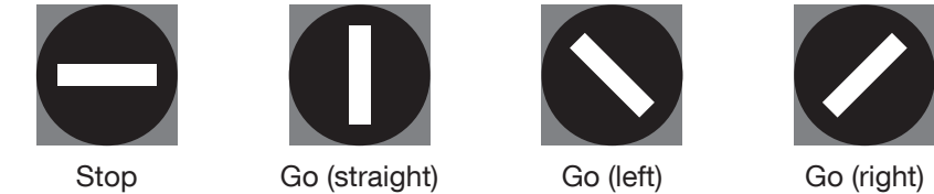
Figure 8D-3. Light Rail Transit Signal Indications
