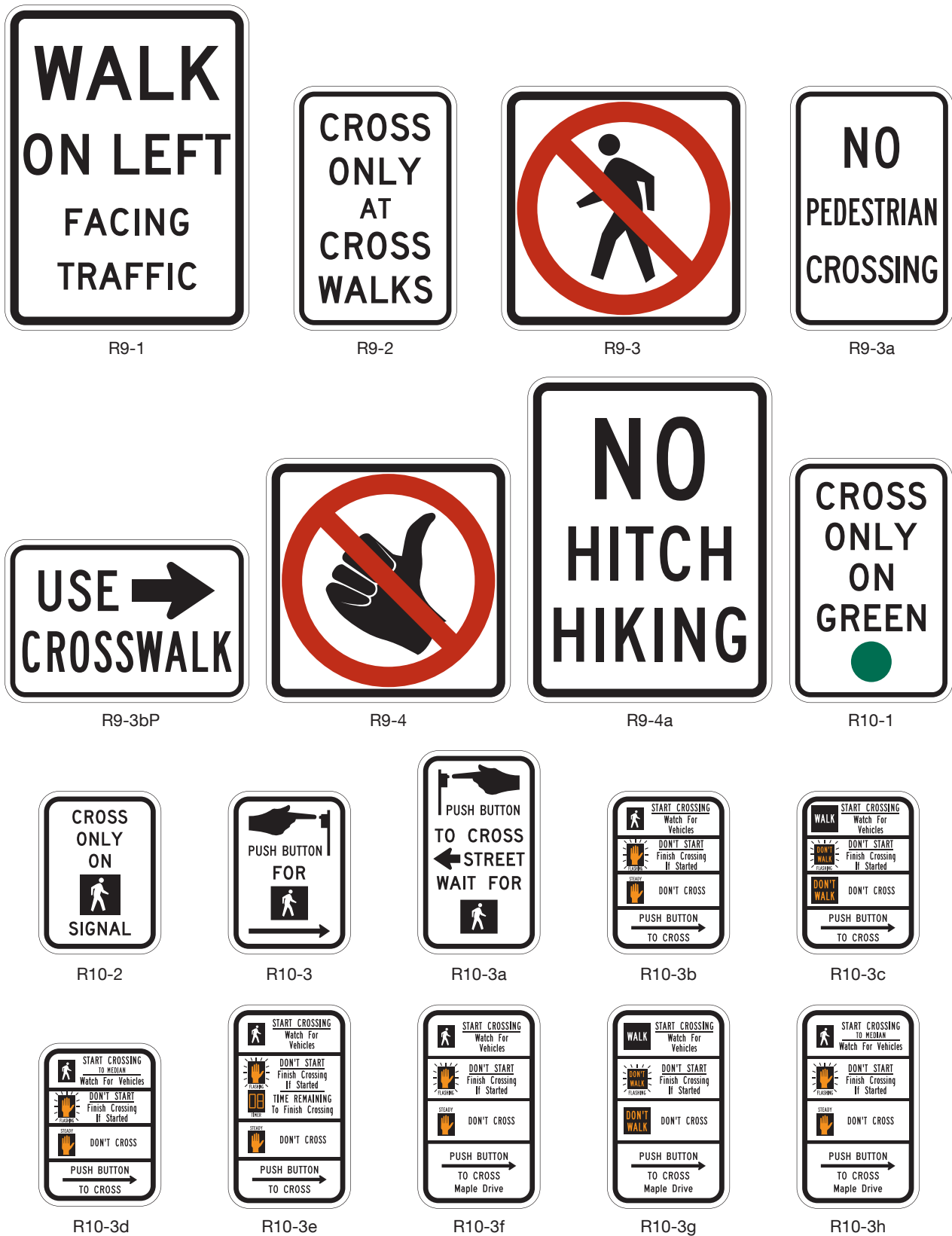
Figure 2B-27. Pedestrian Signs and Plaques (Sheet 1 of 2)
