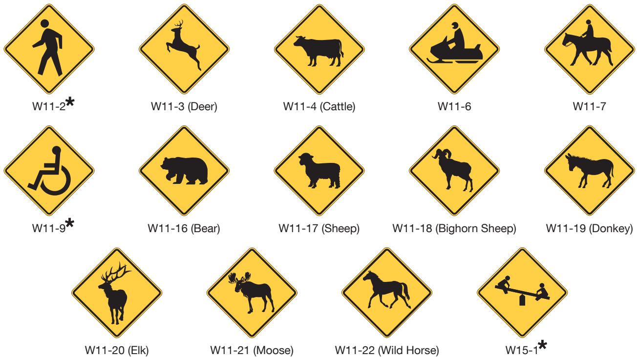
Figure 2C-15. Non-Vehicular Warning Signs
