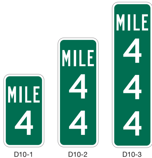
Figure 2H-5. Reference Location Signs
