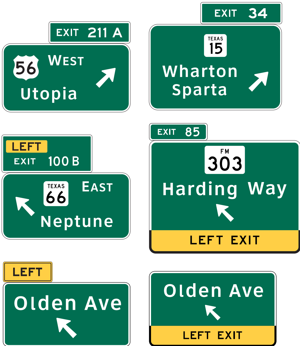
Figure 2E-12. Examples of Exit Direction Signs
