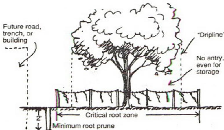
(bb) Tree protection fences located in the development impact area within 15 feet of construction activity must be a minimum of six-feet-high and constructed of chain-link, wire-mesh, or wood fence materials, and be solidly anchored to the ground **if**:
