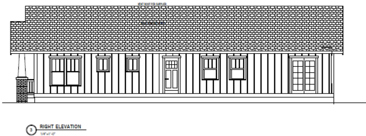
Figure 7 -- Right side elevation. All windows previously approved as wood, one-over-one. Applicant requesting approval for vinyl, multi-light windows.
