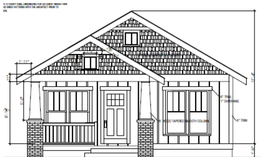
Figure 6 -- Front elevation. All windows previously approved as wood, one-over-one. Applicant plans to keep windows on this elevation as wood, one-over-one.
