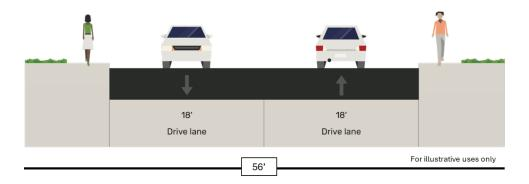
**Existing Operation** – 2-lane undivided roadway in 60 feet of right-of-way and 40 feet of pavement
