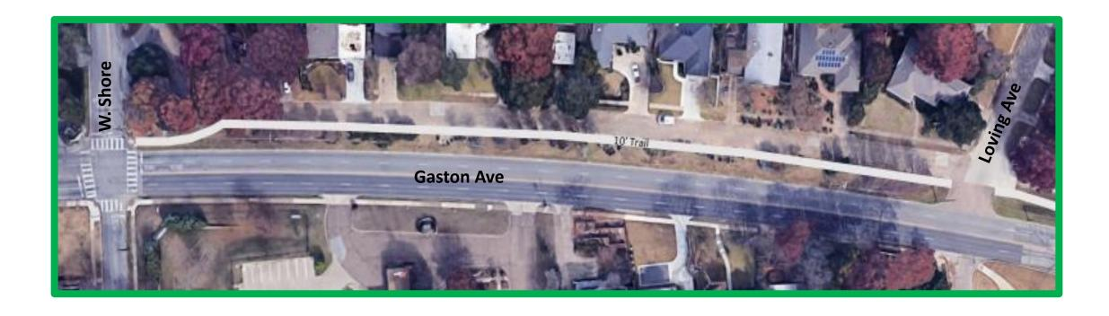
**Draft Recommendation:** 10-foot trail along the north side of Gaston Road between W. Shore Drive and the Santa Fe Trail connection, in the existing right-of-way.
