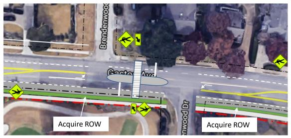
**Draft Recommendation:** A traffic signal is not warranted for this location. Install pedestrian refuge median. Enhance with signage, lighting, and pedestrian signal. Additional right-of-way is needed to construct a wide sidewalk and landscaped buffer.
