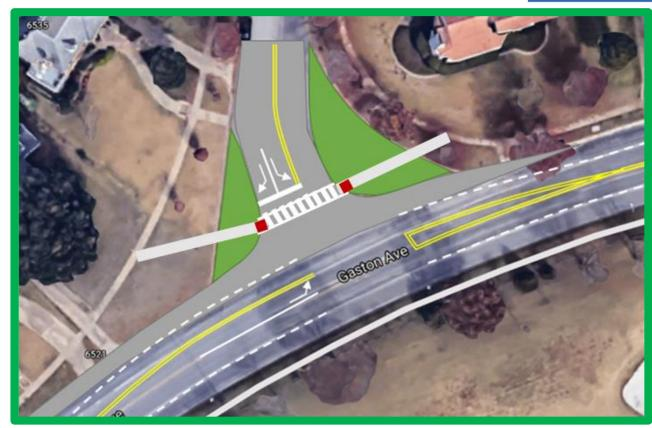
**Draft Recommendation:** There is available right-of-way at the intersection to shift Gaston to install a left turn lane. The existing splitter island at the terminus of Cambria would be removed and the intersection brought to a single point, improving visibility, and slowing turning vehicles entering the neighborhood.
