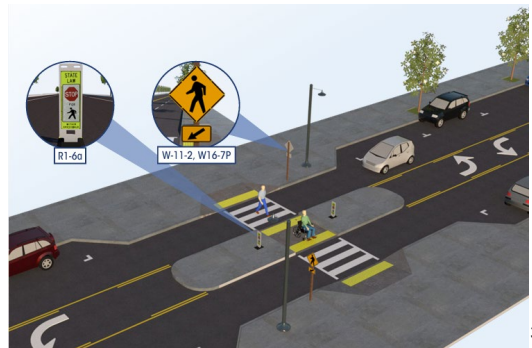
Figure 3: Pedestrian Refuge Island in the Center Turn Lane of a Three-Lane Road
