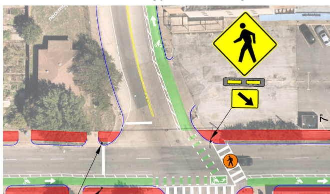
Rectrangular Rapid Flashing Beacon
