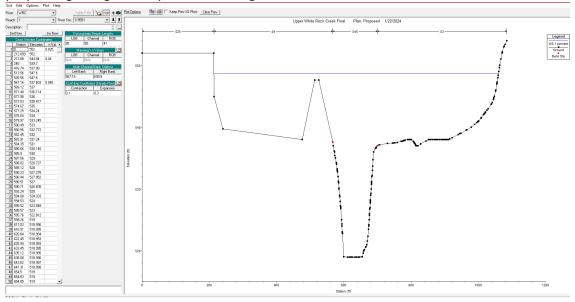
4. In the proposed conditions scenario that includes a pedestrian bridge, the blocked obstruction at cross section 119664 (referenced below) was eliminated. The outcome remained the same.
