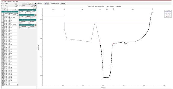
4. In the proposed conditions scenario that includes a pedestrian bridge, the blocked obstruction at cross section 119664 (referenced below) was eliminated. This modeling preference did not alter the final conclusion.
