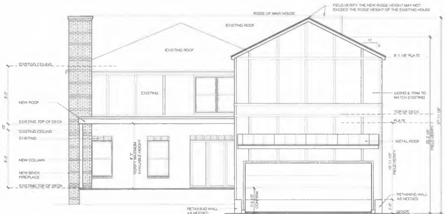
1 REAR ELEVATION SCALE 1/4" = 1'-0"
