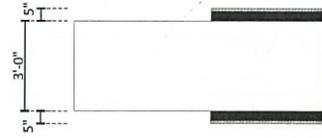
ALUMINUM SIGN CABINET PAINTED WHITE INTERNALLY ILLUMINATED WITH WHITE LED'S WITH FLEX BLEED FACES TO HAVE DIGITALLY PRINTED TRANSLUCENT VINYL OVERLAYS
