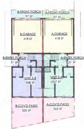
4 1ST FLOOR PLAN 3/32" = 1'-0"
