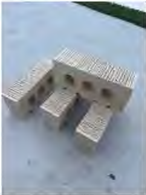
Brick we used to replace broken/cracked bricks throughout the outside. We could not find a matching brick since the original brick was made in 1926.
