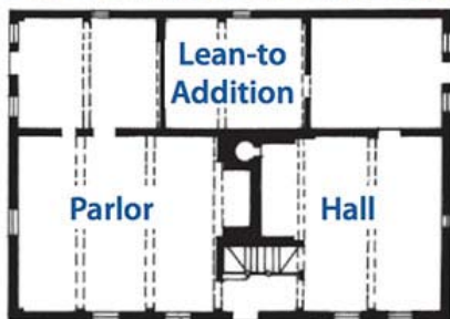
Figure 4. A typical New England saltbox features a steeply sloping roof to shed snow and a floor plan organized around a central chimney to conserve heat.
