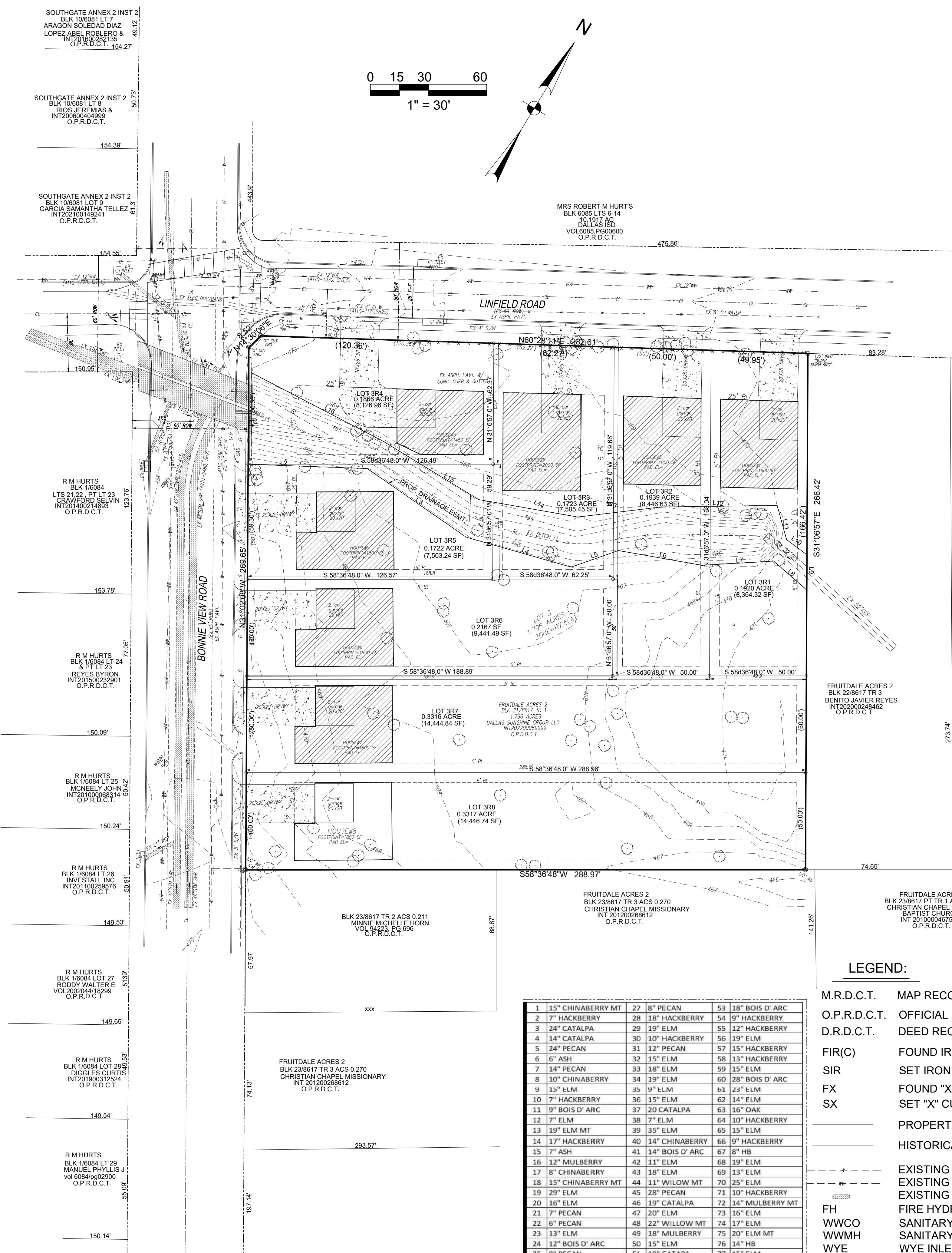
NOTE: THE PURPOSE OF THIS PLAT IS TO CREATE 1 LOT TO 8 LOTS AND PROVIDE EASEMENT FOR THE DITCH COMMON FLOWS.
