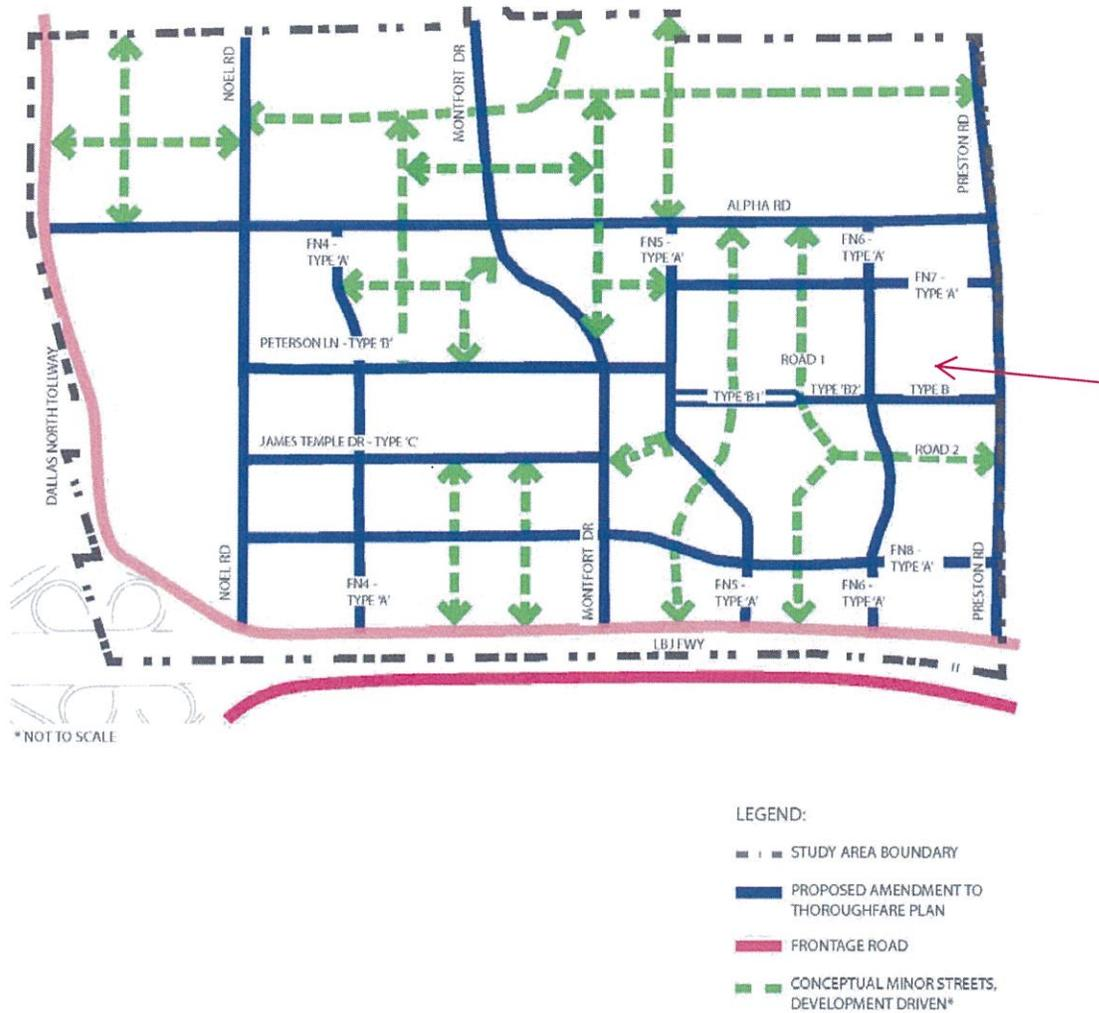
\* THESE MINOR STREETS ARE CONCEPTUAL AND INTENDED ONLY TO ILLUSTRATE DESIRED CONNECTIVITY FOR NEW STREETS. ALTERNATIVE ALIGNMENTS MAY BE APPROVED BY THE DIRECTOR OF PUBLIC WORKS IF THEY PROVIDE EQUIVALENT CONNECTIVITY AND COMPLY WITH THE PROVISIONS OF SECTION 51P-887.115 (STREET STANDARDS) AND SECTION 51A-13.502 (NEW MINOR STREETS).
