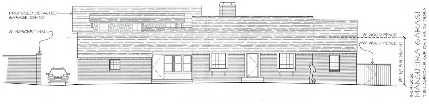
O | SOUTH ELEVATION (FRONT) SCALE: 1/8" = 1'-0"
