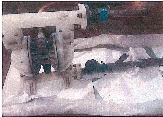
14. Close-up of poly pump used to remove chromic acid waste from sumps.
