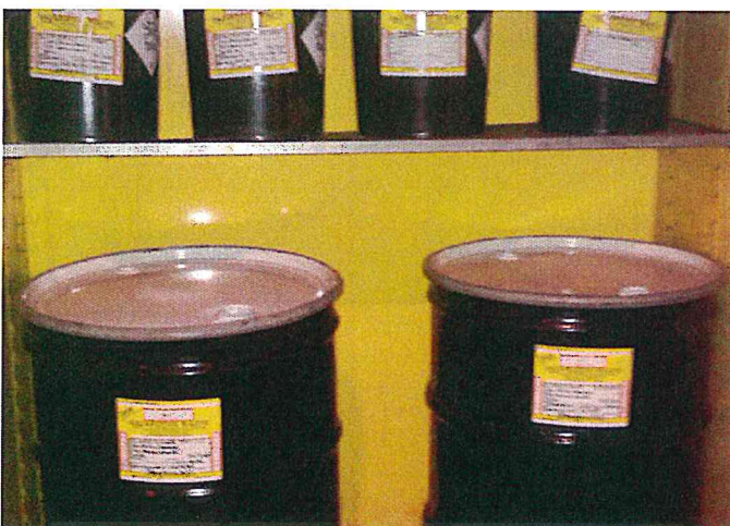
11. View of lab-packed and overpacked containers of cyanide waste secured in cabinet of Lane Plating Facility.
