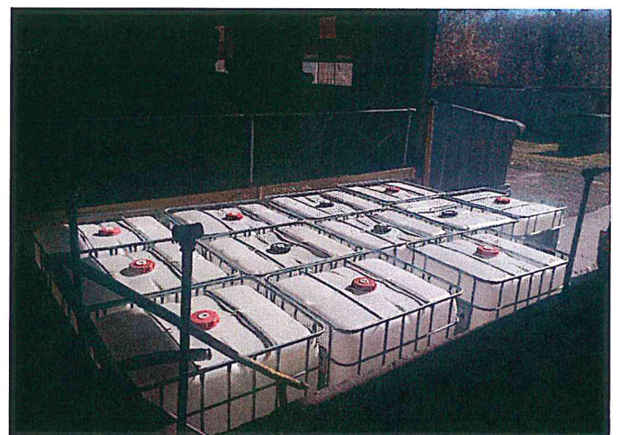
12. View of totes used to store chromic acid waste pumped from sumps at Lane Plating Facility.
