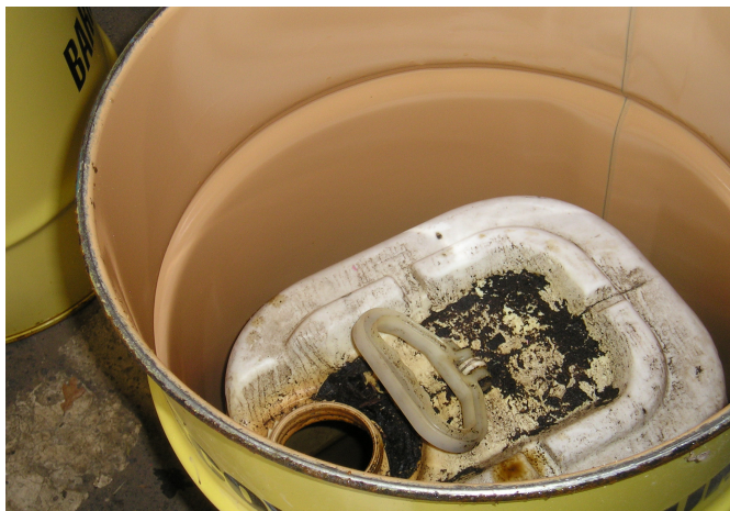
Yes - Place leaking containers into overpack drums
