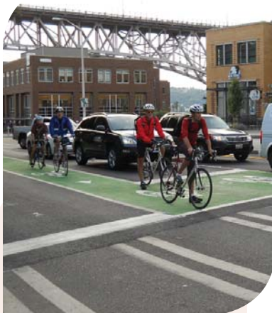
Bicycle box at an intersection
