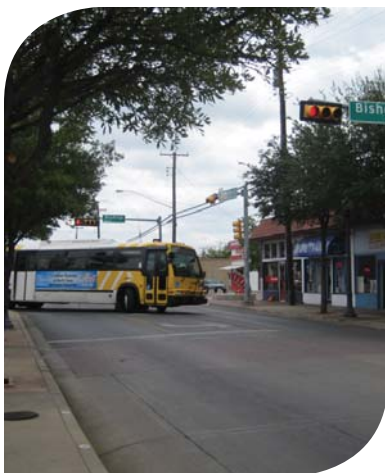
DART buses are up to 40 feet in length, and must be able to navigate intersections.
