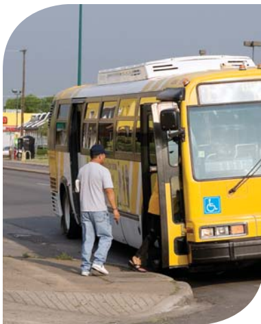
Near-side bus stop on Jefferson Street
