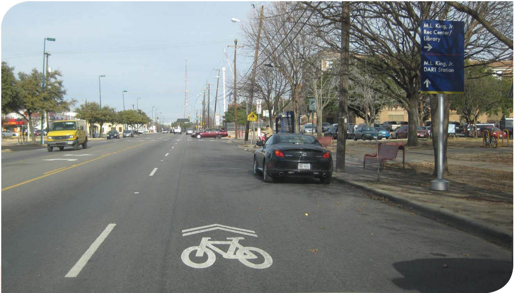
Shared lane markings and wayfinding signage along Martin Luther King, Jr. Boulevard
