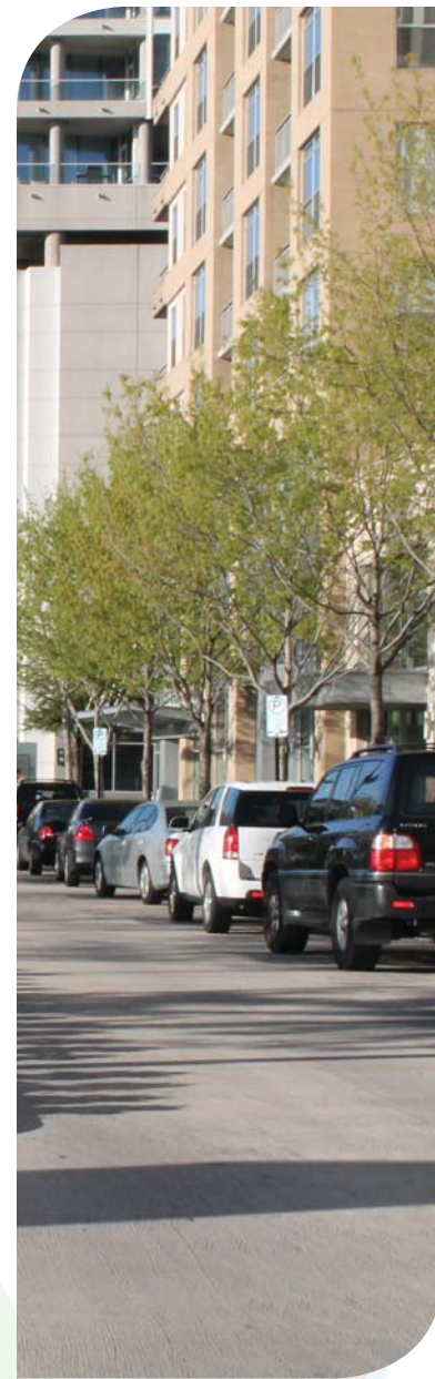
On-street parking creates side friction and reduces vehicle speeds.
