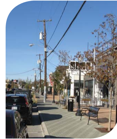
Sometimes existing overhead power lines can remain to serve adjacent property owners and be successfully incorporated into the complete streets design.
