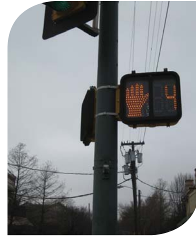
Pedestrian signal with countdown indication
