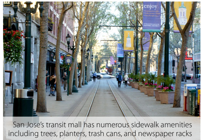
A wide sidewalk, ideally with street trees and lighting, is preferred to protect pedestrians from the adjacent train
