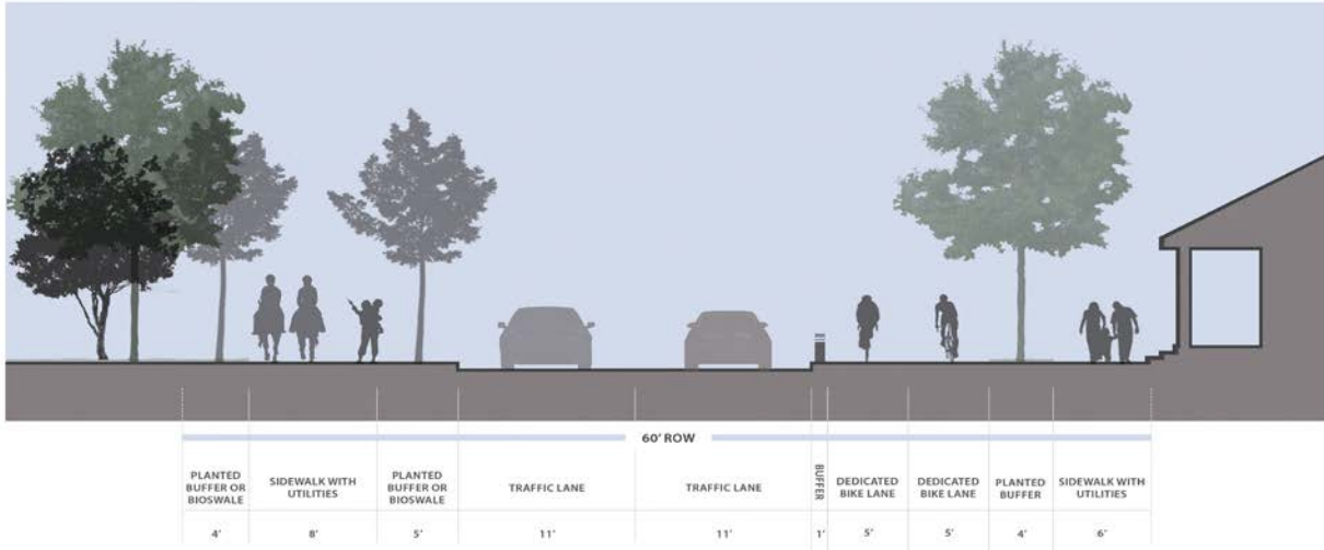
A cross-section design concept for reconstructing the Pemberton Hill Road
