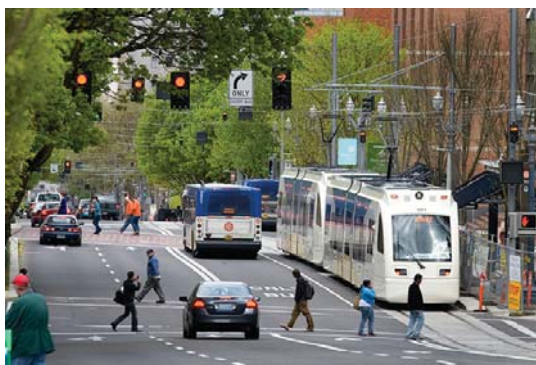
Example of a street which accommodates the pedestrian, bicycle, public transit, service vehicles, and the private vehicle
