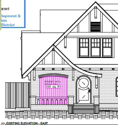
① EXISTING ELEVATION - EAST 1/4" = 1'-0"
