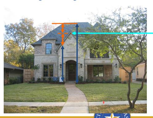
Height is a horizontal plane measured ½ way between peak and eave.
