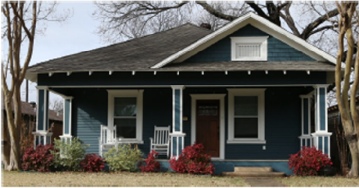
Examples: Recessed gable above the front porch.
