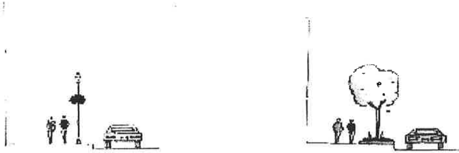
Figures 1 & 2: Examples showing various techniques to provide horizontal separation between pedestrian and vehicular traffic.
