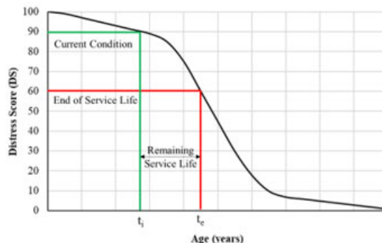
Figure 3. Sample Deterioration Curve
