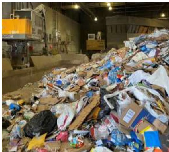
Figure C-6: Recyclables Stored in Front of Direct Load Hopper at Bachman Facility
