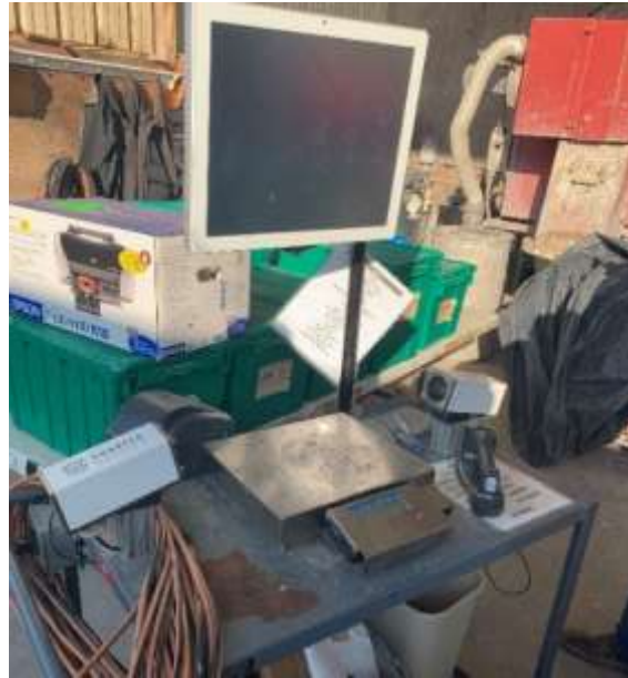
Figure 12-3: Smarter Sorting Scanning and Weighing Equipment
