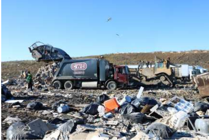
Figure E-13: Conventional Collection Vehicle Ejecting Material on Tipping Deck
