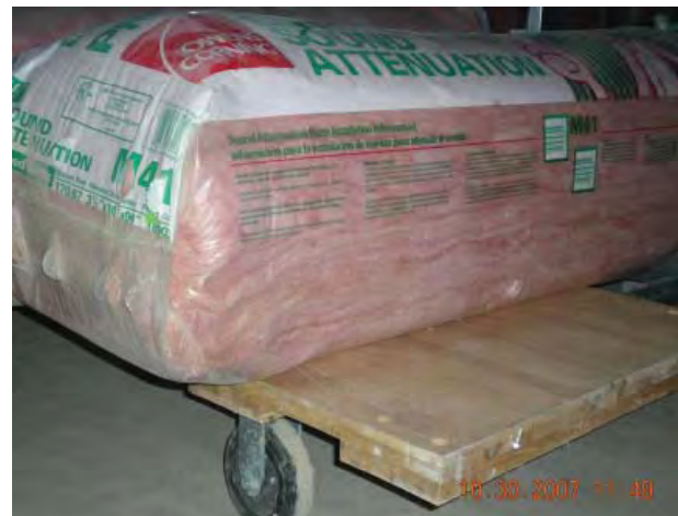
Insulation Wrapped and Protected From Moisture.
