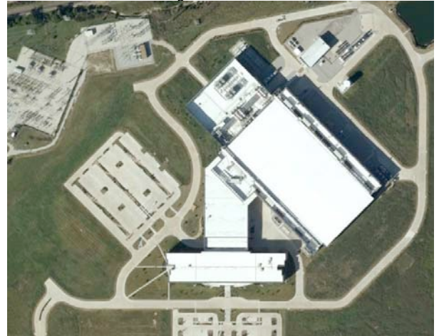
Figure R5: The Texas Instruments RFAB facility in Richardson, Texas used reflective roofing as well as reflective building and paving materials to achieve urban heat island mitigation benefits.
