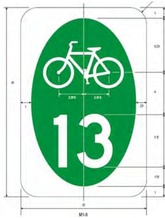
Figure 28. Regional route sign.
