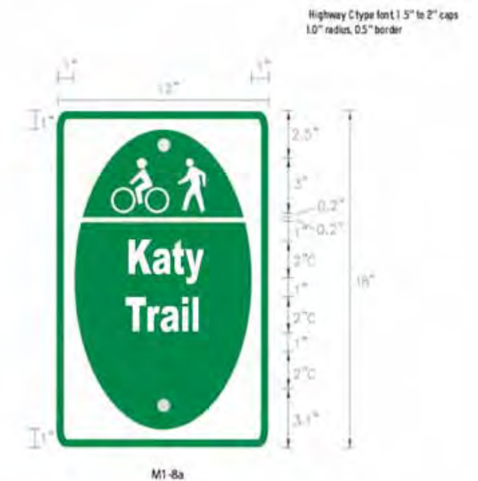
Figure 27. Regional route sign.
