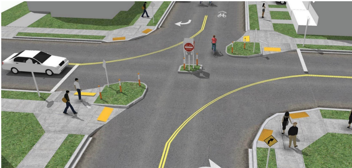
FIGURE 8: DIAGONAL DIVERTER (SOURCE: NACTO)
