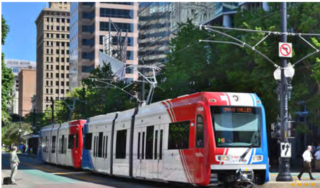
Catenary poles and wiring should incorporate street lighting and be aesthetically appealing
