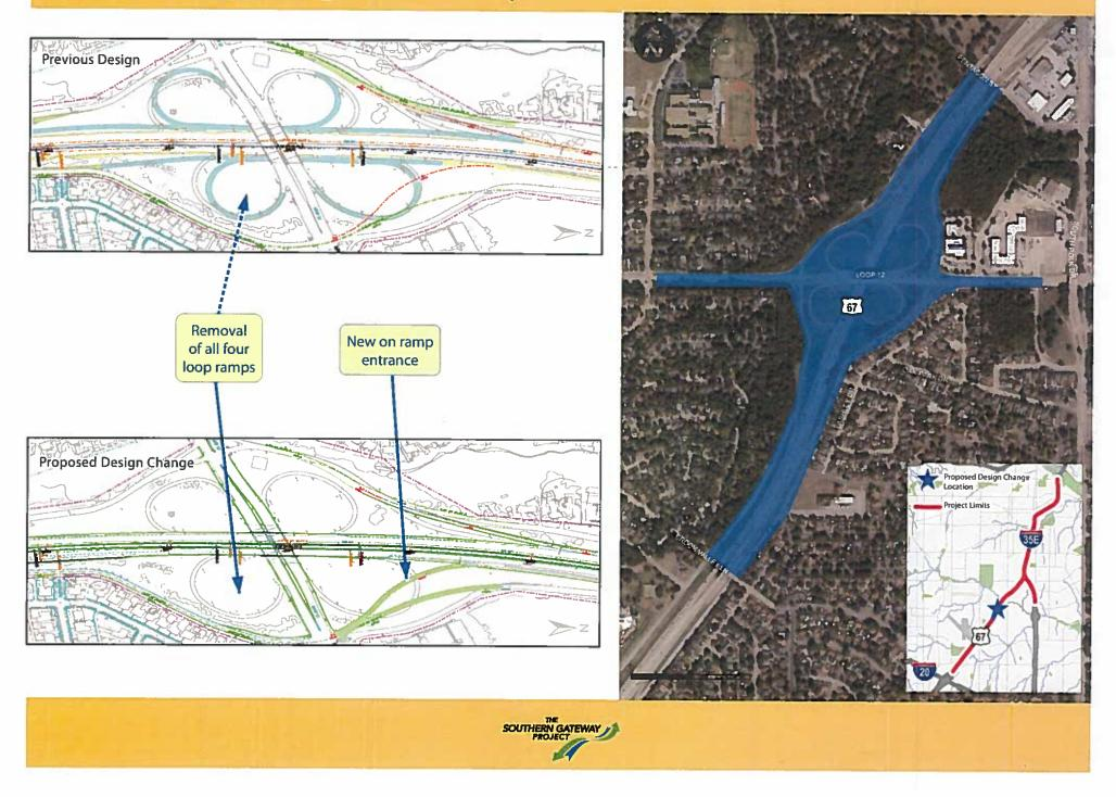
MODIFICATIONS PROPOSED FOR A SECTION OF THE I-35E/US 67 PROJECT AT LOOP 12
