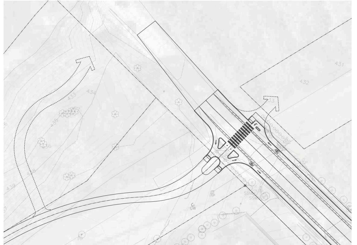
Trail spur connects seamlessly into new Highland Road Complete Street design; also designed for future Ash Creek Greenbelt Trail
